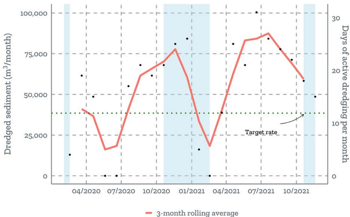
Figure IV.11. Kapichira dredge activity and sediment removal volumes by month
