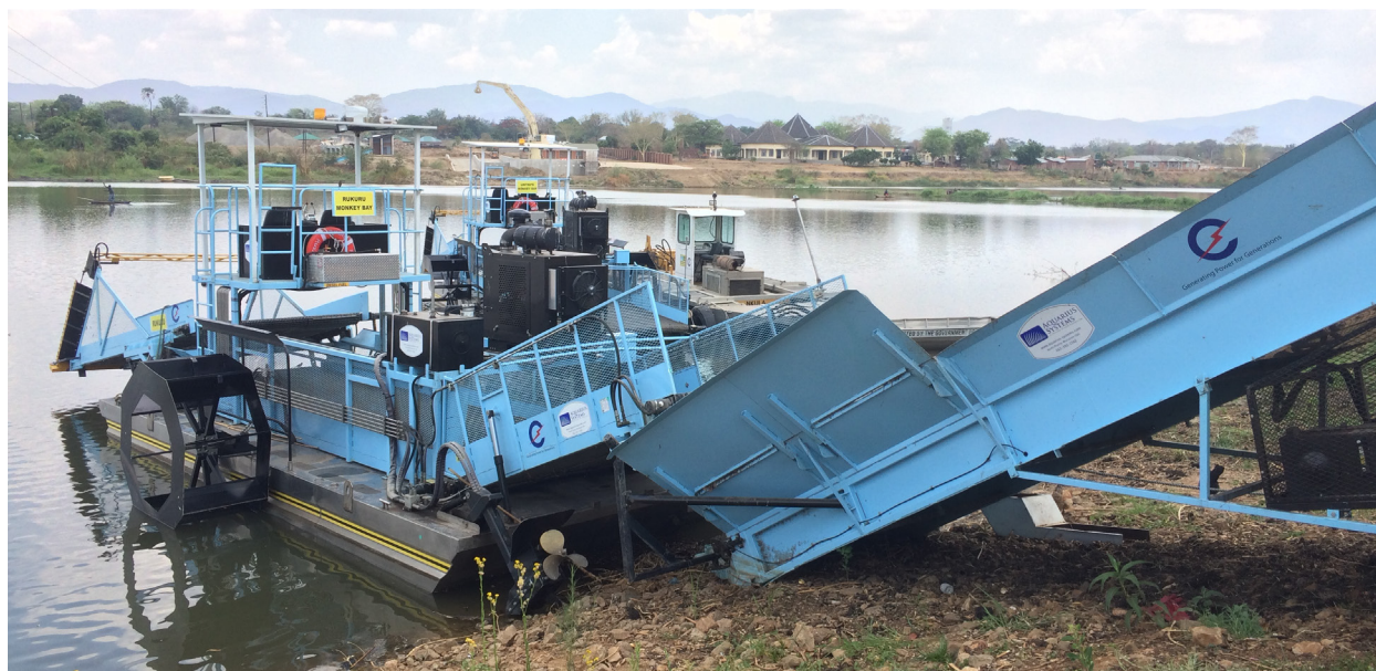
Figure IV.3. Weed harvesters and conveyor belt procured under the WSM activity (Liwonde barrage)
