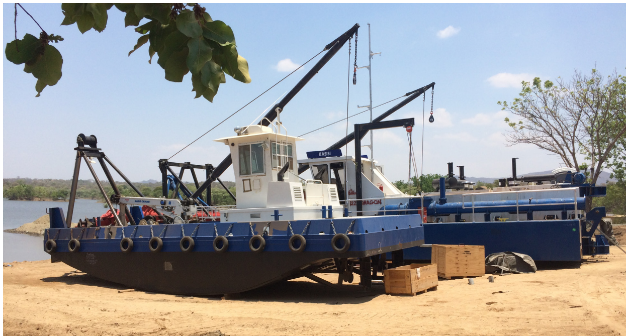
Figure IV.8. Newly procured dredging equipment (Kapichira power station)
