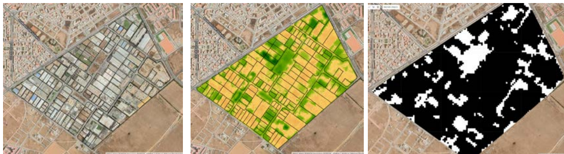
Figure VI.1. Example of using remote sensing data to detect undeveloped land
