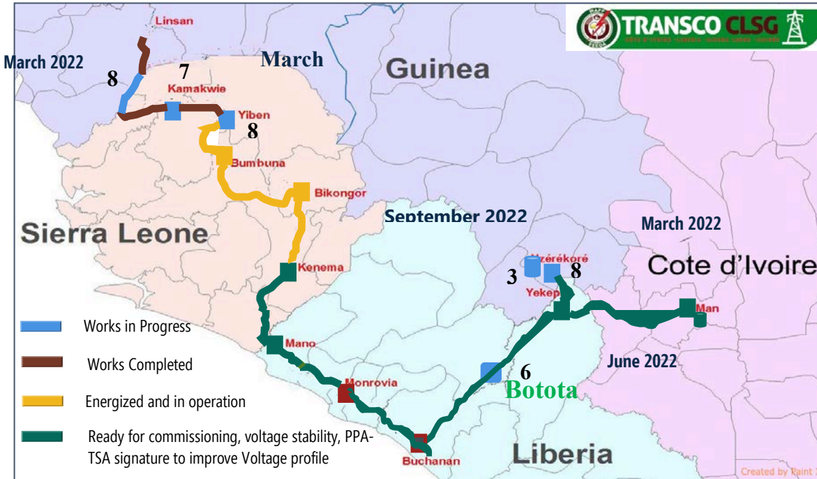
Figure V.17. CLSG Transmission line (Transco) and project details (PPA and TSA)
